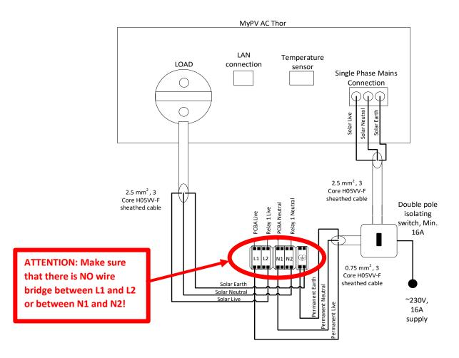
**Note**: Heat Battery Controller Connection above only shows Power Terminal connections, for other Heat Battery wiring, please reference to Installation Manual provided with Heat Battery.
