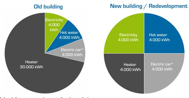
**Rule of thumb for power requirements for photovoltaics:** Hot water & space heating in residential buildings: min. 3 kWp / residential unit Hot water: 1.5 kWp / residential unit (2 or 3 residents); 2.0 kWp / residential unit (4 to 6 residents)
