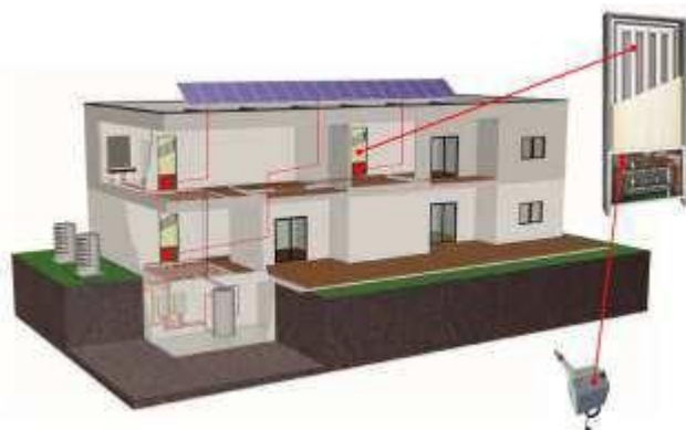
Example for hot water wall-integrated storage, copyright: Pink GmbH
